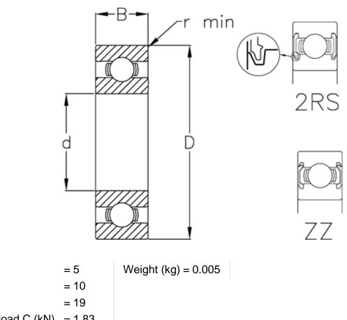
D = 19 Dynamic load C (kN) = 1.83 Max rpm greased = 32000 Max rpm oil lubricated = 38000 r min = 0.3 Static load C0 (kN) = 0.93
